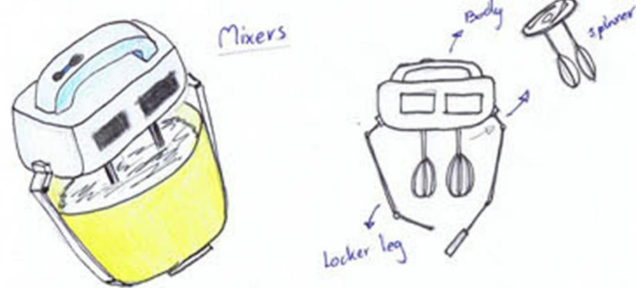
Many mixers has base on its but it is not suitable for carrying. This machine got shaky when using it so I decide to make it hand-using so you have to control by yourself but I did put locked for locking container.
