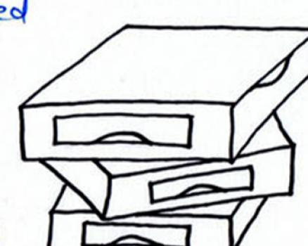
In my final design, compared to my original I have developed a draw that the user can open and have the toast cooked in. I designed handles for the draws as well as handles on the side of the top and middle sections so the user can twist them to their desired position.
