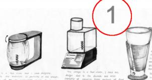
If allows the users to open the cover a little harder, but it gives a secure to them. The users need to remove the safety first and then turn the cover cluck - direction to separate from the container.
